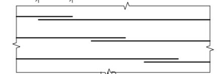
TYPICAL CONSTRUCTION JOINT IN VERTICAL WALL LAP LENGTH 'LH' ELEVATION : X LAP LENGTH LH : 1.0xL FOR HORIZONTAL STEEL
